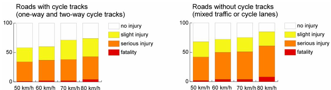
*Cycle tracks physically separated from the roadway give the best protection of cyclists at roads with a speed limit of 50 km/h or more (ref 1, page 42).*
